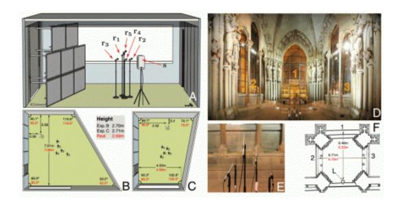
(A) Illustration of the room used in the experiment with a movable wall. (B and C) Two reconstruction results. Real values are indicated in red, and the estimated values are indicated in black. (D) Panoramic photo of the portal of the Lausanne cathedral. (E) A close up of the microphone array used in cathedral experiments. (F) Floor plan of the portal. Credit: (c) PNAS, DOI: 10.1073/pnas.1221464110
