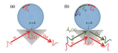
In a whispering-gallery-mode resonator, a photon could become so intense that it produces a nonlinear effect, enabling quantum gates. Reprinted with permission, Yu-Zhu Sun, Yu-Ping Huang, and Prem Kumar, *PRL* 110, 223901 (2013).
