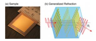
(a) Photograph of an ultrathin (72 µm thick) metamaterial sample.
