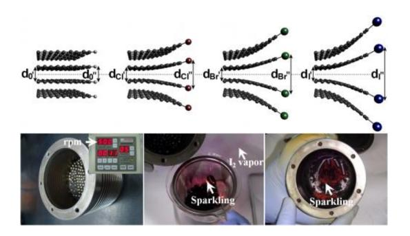
A schematic representation for the edge expansions of XGnPs is seen in the top images. The bottom images contain ball-mill capsule containing the pristine graphite and stainless steel balls. Credit: UNIST
