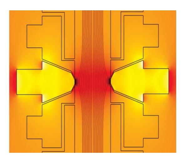
A Penning trap with a 'magnetic bottle' magnetic field in which single protons can be captured for several months. The magnetic field lines of the trap are shown. Credit: 2013 Stefan Ulmer, RIKEN Ulmer Initiative Research Unit
