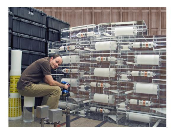
Larry Hudson with NIST-fabricated examples of test artifacts called out by the new CT image quality standard for security applications.
