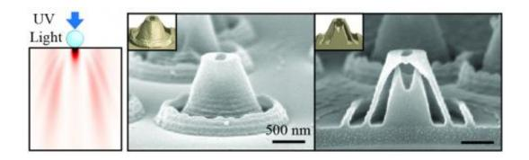
Researchers from NC State University are able to carve nanoscale "volcanoes" by scattering light through a polymer "crystal ball" onto a photo-reactive thin film. The structures hold promise for new drug-delivery technologies. Credit: Chih-Hao Chang, North Carolina State University
