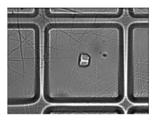
A 10 micron crystal placed, using laser light, onto a 50 micron square aperture backed with microfibres ready for freezing and X-ray diffraction studies.
