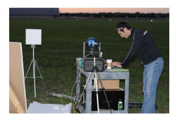
Joseph Meola of Air Force Research Labs conducting measurements on laser light bounced back from various samples placed 1.6 kilometers on the ground from a prototype laser at Wright Patterson Air Force Base. Credit: Anthony Absi, Air Force Research Labs
