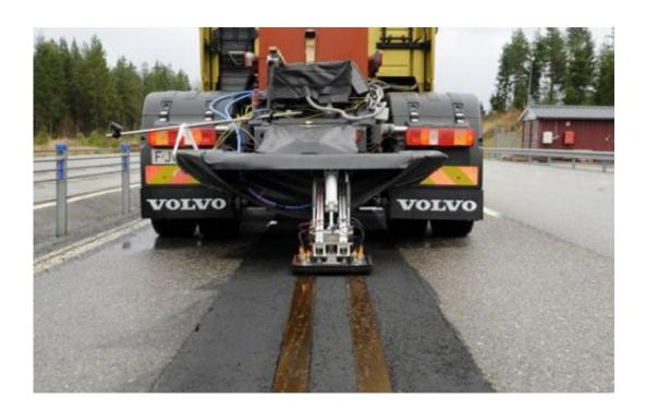
(Phys.org) —How are engineers doing in solving the problem of large-sized all electric transport vehicles traveling long distances without the burden of large batteries? One workaround that has been the topic of much discussion is the use of power lines that are built into the surface of the road. The Volvo Group has issued its state of progress and says it has come a long way in its research but that there's still work and planning decisions ahead. The goal is to find a cost-efficient way to
