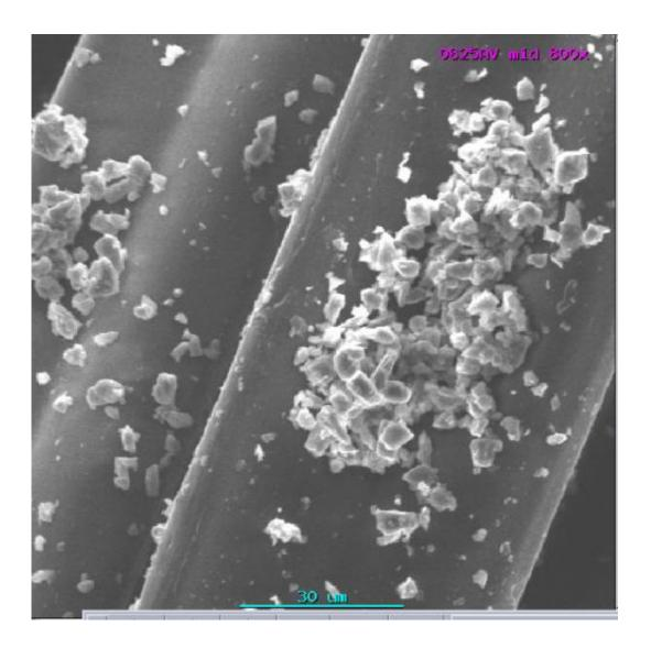
This is a microscope image of rug fibers with deposited test particles. Credit: Andrea Ferro, Clarkson University
