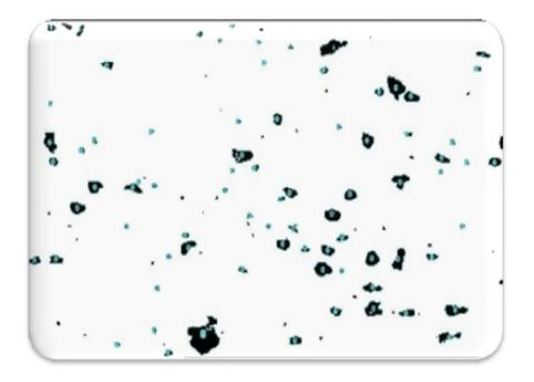
Image of particles on flooring surface. Particles are sized and counted using the National Institutes of Health imaging software. Credit: Andrea Ferro, Clarkson University
