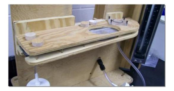
Basic wind tunnel apparatus. Floor samples seeded with particles are placed in test section and images of the particles on the flooring surface are taken over time. The images are analyzed to determine relationship between particle detachment and friction velocity. Credit: Andrea Ferro, Clarkson University
