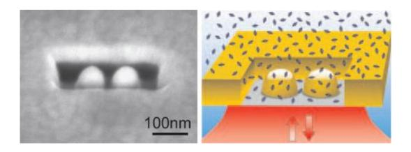
This is a dimer antenna inside a nanobox for single biomolecule analysis at high concentrations. Credit: ICFO
