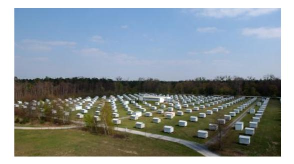
The KASCADE-Grande measurement field on the premises of KIT was used by scientists to study particle showers produced by cosmic rays. Credit: KIT
