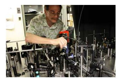
NIST physicist Alan Migdall spotlights the crystal that converts one photon to two in the middle of the complex apparatus used as a high-efficiency source of paired photon for quantum experiments. Credit: Baum/NIST
