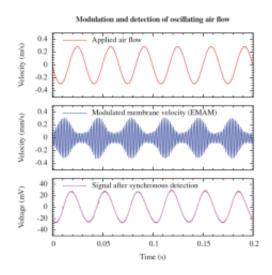
The original signal (top), the signal at a sensor vibrating at a higher frequency (centre), and the reconstructed signal (bottom).
