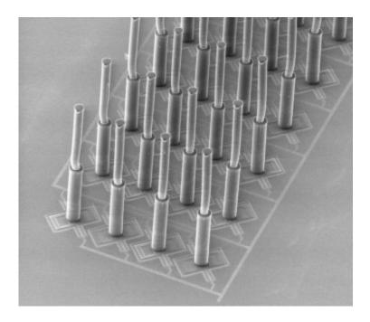
Tiny "hairs" of the polymer SU-8 are applied to a flexible, moving surface, the capacitance of which changes with each movement.
