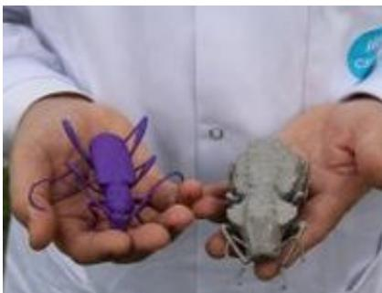
Up close and personal with the CSIRO printed titanium bugs.
