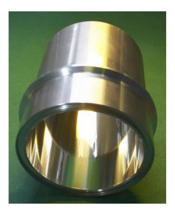
Precision boring of cylinder running surfaces rely on defined cuts with a specific geometry. Thus, surfaces of a very high quality can be created. Credit: Fraunhofer IWU
