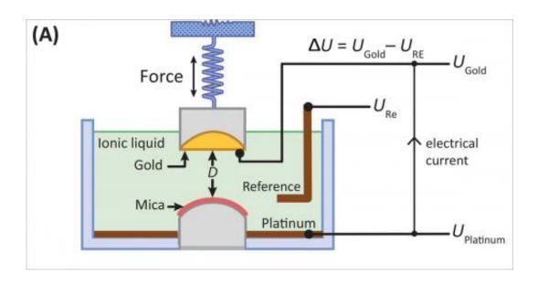
This is a diagram of the surface forces apparatus used to study ionic liquids. Credit: Matthew Gebbie
