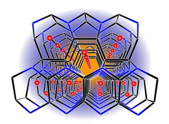
A newly synthesized borosilicid framework hosts lithium atoms in its channels, making it a promising candidate for electrodes of lithium-ion batteries. Credit: T. Faessler/M. Zeilinger, Technische Universitaet Muenchen
