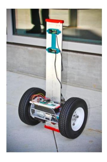
FFR is a robotic scout for firefighters developed by the Coordinated Robotics Lab at UC San Diego. Credit: Jacobs School of Engineering/UC San Diego
