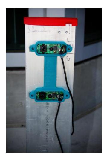
FFR is equipped with stereo cameras that allow the robot to create 3-D imaging maps. Credit: Jacobs School of Engineering/UC San Diego
