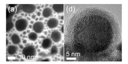
Transmission electron microscopy (TEM) images of the gold-indium alloy nanoparticles at room temperature. (A) shows an overview of multiple particles, while (D) shows a high-resolution TEM image of one nanoparticle's crystalline gold-indium core surrounded by the amorphous and catalytic oxide shell.
