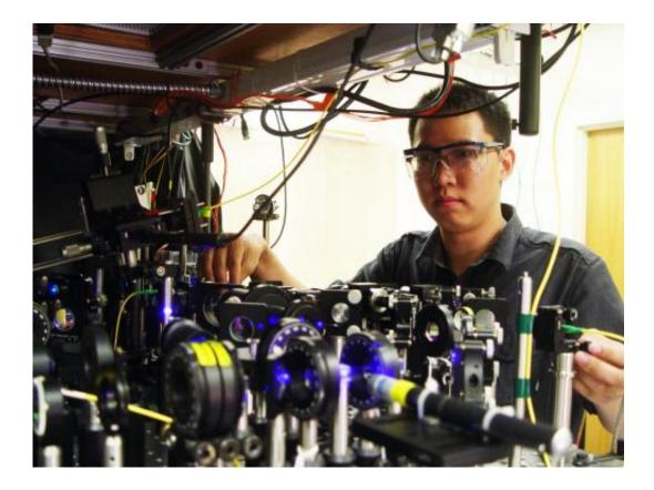
Georgia Tech graduate student Lin Li adjusts the optics on equipment being used to measure the entanglement between light and an optical atomic excitation in the laboratory of Alex Kuzmich. Credit: Kuzmich Physics Lab
