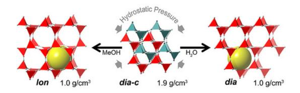
Pressure-induced transitions are associated with near 2-fold volume expansions. While an increase in volume with pressure is counterintuitive, the resulting new phases contain large fluid-filled pores, such that the combined solid + fluid volume is reduced and the inefficiencies in space filling by the interpenetrated parent phase are eliminated.
