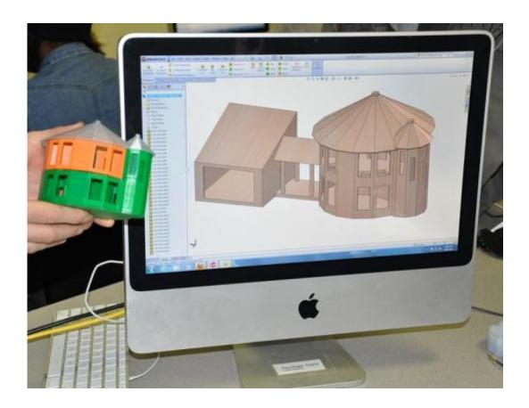
Eric Lipsky, an assistant professor of mechanical engineering at Penn State Greater Allegheny, allowed students to print a 3-D model of a Zero-Emissions Home they designed for a class project. Students modeled the house using CAD software, which helps to visualize their designs as they can rotate it and see different views of the design on the computer screen. Credit: PENN STATE
