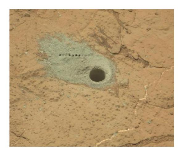
The Chemistry and Camera (ChemCam) instrument on NASA's Mars rover Curiosity was used to check the composition of gray tailings from the hole in rock target "Cumberland" that the rover drilled on May 19, 2013. Credit: NASA/JPL-Caltech/MSSS
