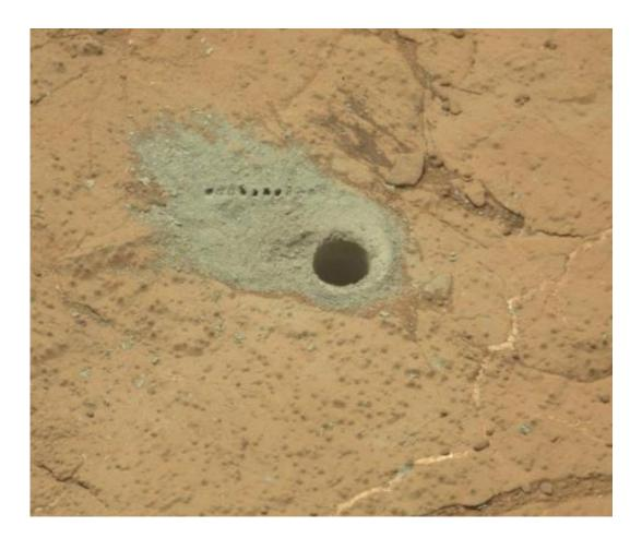
The Chemistry and Camera (ChemCam) instrument on NASA's Mars rover Curiosity was used to check the composition of gray tailings from the hole in rock target "Cumberland" that the rover drilled on May 19, 2013. Credit: NASA/JPL-Caltech/MSSS
