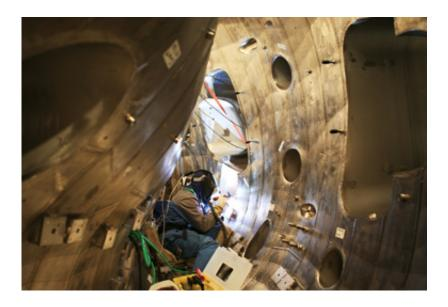
Precision work: One of over 250 ports being brazed in the plasma chamber. Credit: IPP, Anja Ullmann
