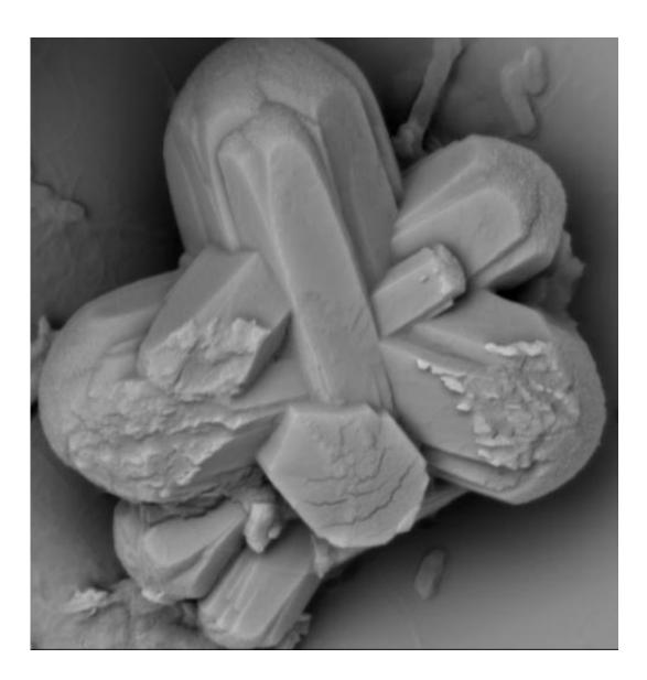
This is a Scanning electron microscope image of calcium carbonate crystals grown in artificial seawater containing individual coral acidic protein (CARP3). These crystals were formed both in pH 8.2 and 7.6. The reticulate structure of
