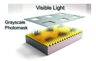
(Phys.org) —Polymer brushes are polymers in which individual polymer chains stand side by side on a surface, causing the chains to stick out like bristles on a brush. In the journal *Angewandte Chemie*, American scientists have now presented a new simple method for making threedimensional nanostructures in a controlled fashion from polymer brushes.
