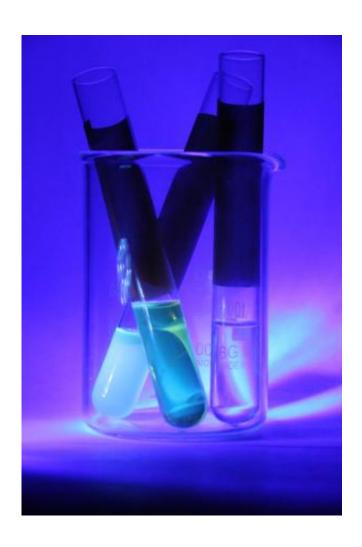
This image shows novel cadmium selenide (CdSe) quantum dots with ligand enhancement chemistry. The vials on the left contain quantum dots; the vial on the right contains solvent without quantum dots. Credit: Delaina Amos.
