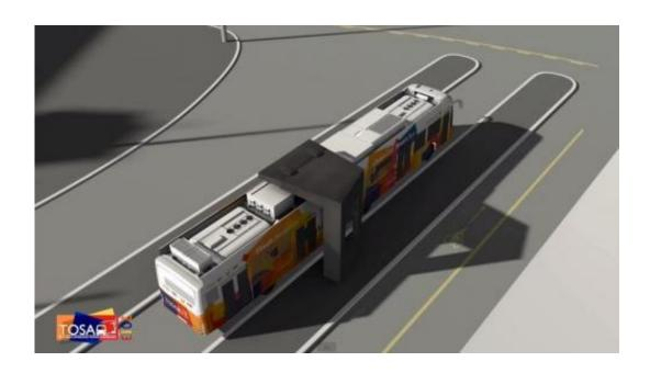
(Phys.org) —A new type of battery bus system being tested in Switzerland is able to operate continually by making use of flash-charging stations. Called Trolleybus Optimisation Systeme Alimentation (TOSA), the new bus and recharging system is currently being tested on a one mile route in Geneva between the city's airport and international exhibition center.
