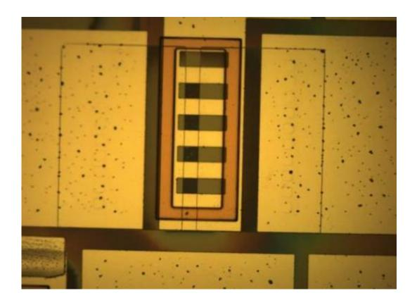
A silicon circuit, coated with a protective layer and immersed in fluid that mimics human body chemistry. Researchers at The Ohio State University are developing low-cost electronic devices that work in direct contact with living tissue inside the body. Credit: Ohio State University.
