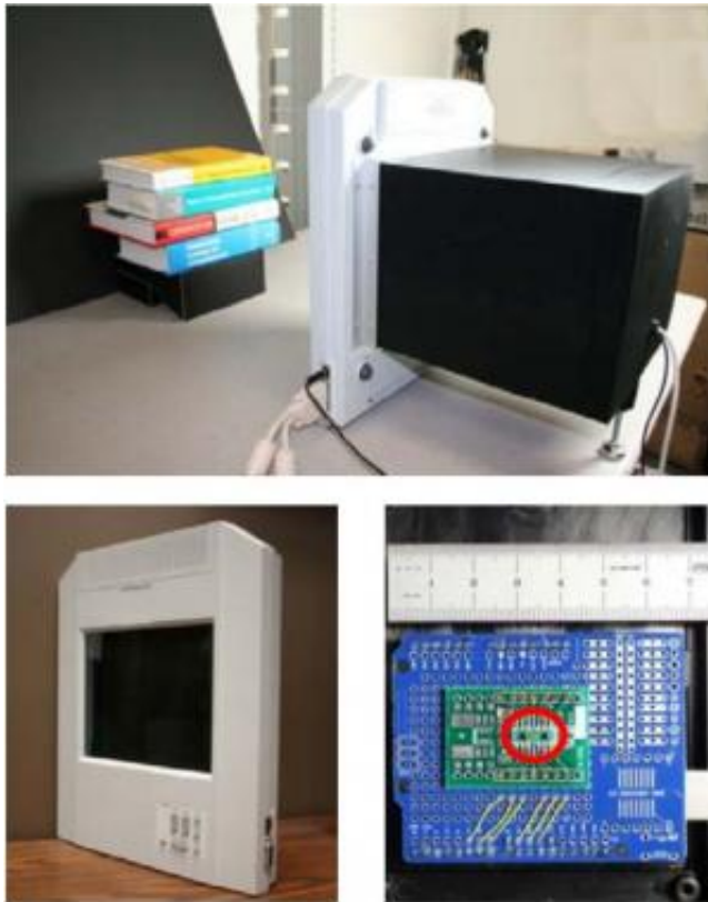
Prototype device. Top: lab setup. Bottom left: the LCD screen as the aperture assembly. Bottom right: the sensor board with two sensors, indicated by the red circle. Credit: arXiv:1305.7181 [cs.CV]
