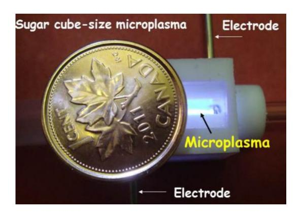
Battery-operated sugar-cube-size microplasma: The microplasma fits inside the letter "A" of a one-cent coin (shown for scale); the sample is introduced into the chamber to the right. Credit: Vassili Karanassios, University of Waterloo
