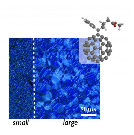
This is the optical microscopy image of a layer of PCBM, a fullerene used in solar cells first synthesized at UC Santa Barbara by Fred Wudl, with (small) and without (large) the nucleating agent. The small domains form in the presence of the nucleating agent, demonstrating the new ability to control the size of crystallites of PCBM. Credit: UCSB
