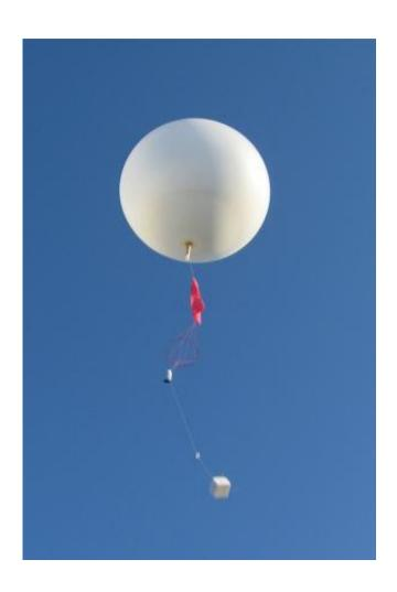
This image shows a weather balloon on its voyage to the upper atmosphere. Launched once or twice a day from stations throughout the world, balloons are used to measure wind speed and direction up to 19 miles high. Credit: Cliff Lawson, Radiosonde Museum.
