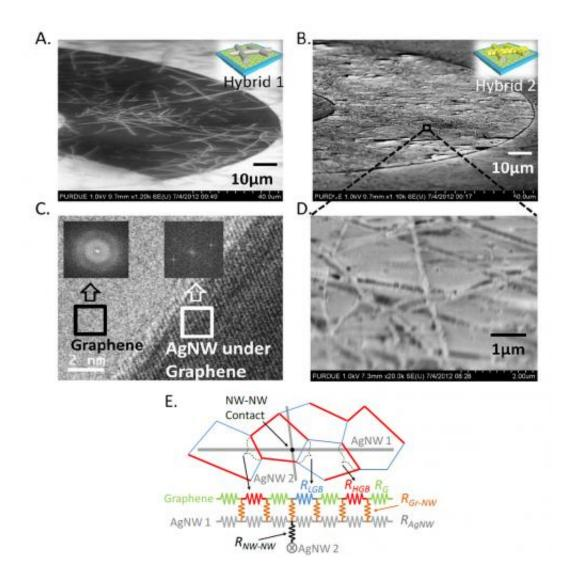
These electron microscope images show a new material for transparent electrodes that might find uses in solar cells, flexible displays for computers and consumer electronics, and future "optoelectronic" circuits for sensors and information processing. The electrodes are made of silver nanowires covered
