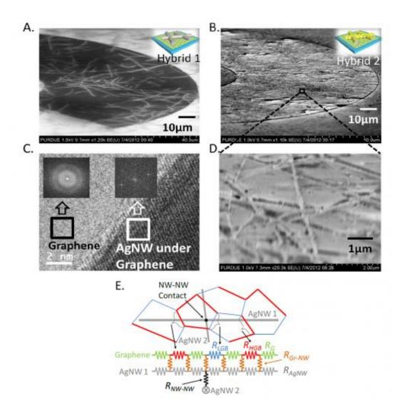
These electron microscope images show a new material for transparent electrodes that might find uses in solar cells, flexible displays for computers and consumer electronics, and future "optoelectronic" circuits for sensors and information processing. The electrodes are made of silver nanowires covered
