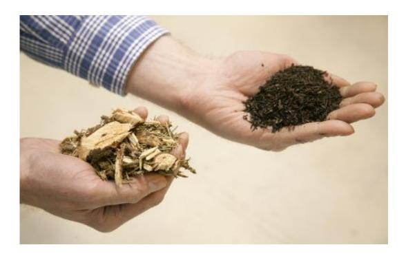
Torrefaction concentrates the energy content of biofuels. Left: chopped-up branches and tops. Right: this type of raw material has been subjected to torrefaction before being ground into a fine-grained mass, which is then pressed into pellets. This contains about 70 per cent of the original mass, while keeping 90 per cent of its energy.
