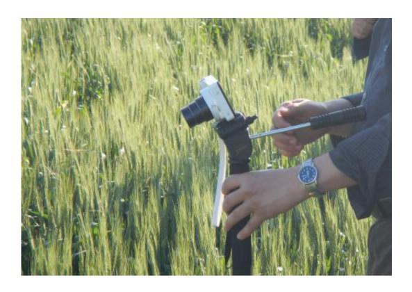
This "smart" camera is part of a computerized system designed to provide early pest detection in wheat fields. Credit: Oregon State University
