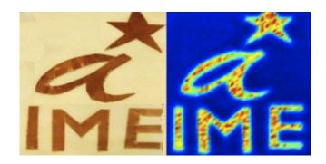
Terahertz radiation can penetrate materials such as a paper envelope and reveal the contents (left) in an accurate image (right). Credit: 2013 A\*STAR Institute of Microelectronics
