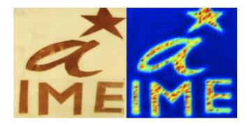
Terahertz radiation can penetrate materials such as a paper envelope and reveal the contents (left) in an accurate image (right). Credit: 2013 A\*STAR Institute of Microelectronics
