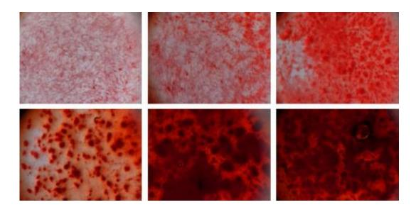
Silicate nanoplatelets cause stem cells to become bone cells, as determined by the formation of bone matrix (in red). Credit: Khademhosseini lab
