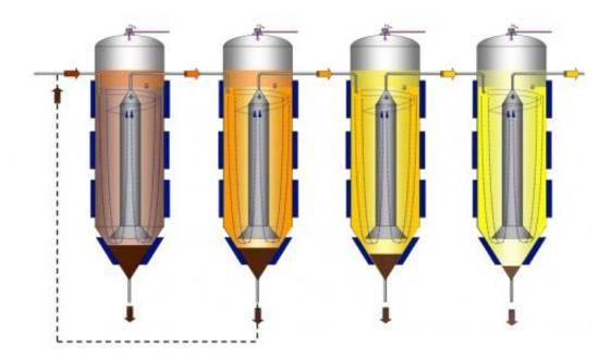
Non-stop fermentation: The product constantly flows from left to right. All tanks are permanently filled during the complete operation time, which in this case is at least several weeks or months. Sediments like yeasts can be reused efficiently as desired. Credit: K. Auffermann-Müller/TUM
