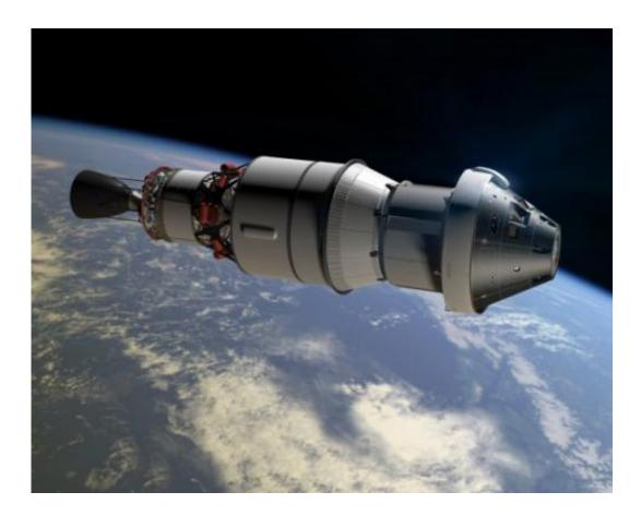
An artist concept shows Orion as it will appear in space for the Exploration Flight Test-1 attached to a Delta IV second stage. Credit: NASA
