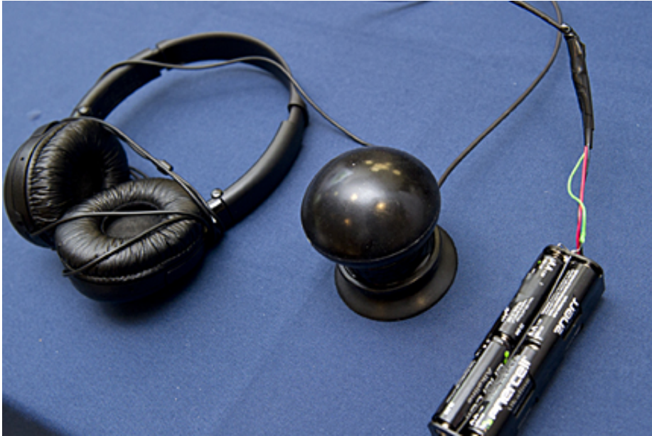
Components for a space stethoscope. Credit: Will Kirk/homewoodphoto.jhu.edu
