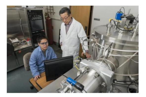
UD professor John Xiao (standing) and research associate Xin Fan work with the high vacuum magnetron deposition system, which is used to fabricate layered thin films in a vacuum for spintronics research. Credit: Evan Krape/University of Delaware
