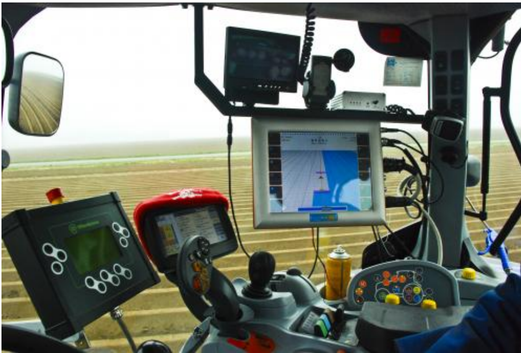
Tractor guidance system. Credit: Navtronics BVBA
