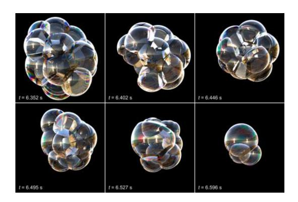
Snapshots from a multiscale model of membrane rearrangement, drainage and rupture in a cluster of soap bubbles, shown using thin-film interference. Credit: Saye & Sethian, UC Berkeley/LBNL
