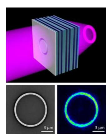
Bottom left: Scanning electron micrograph of a ring-shaped opening in a chromium sheet located on the surface of a flat slab of metamaterial. Bottom right: Optical micrograph of the image projected beyond the slab under UV illumination, demonstrating that the metamaterial slab acts as a flat lens. Credit: Lezec/NIST
