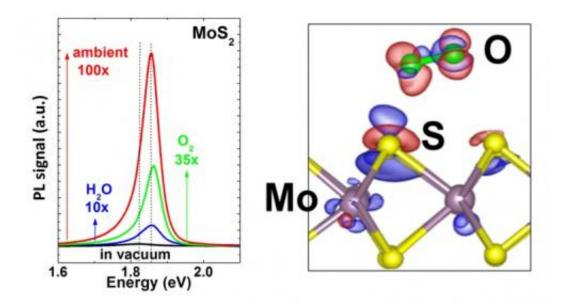
(Left) Graph showing the change in photoluminescence of MoS2 upon exposure to H2O alone, O2 alone, and ambient air at pressures of 7, 200, and 760 Torr, respectively. (Right) Figure showing the charge density difference between pristine MoS2 and O2-adsorbed MoS2. Credit: Sefaattin Tongay, et al. ©2013 American Chemical Society
