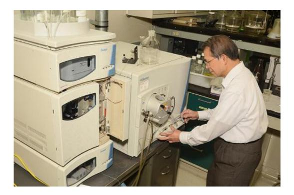
A protocol developed by chemist Ken Lin helps to simplify the use of ESI-MS (electrospray ionization mass spectrometry) to determine whether an olive oil sample contains oil other than that extracted from olives. Credit: De Wood
