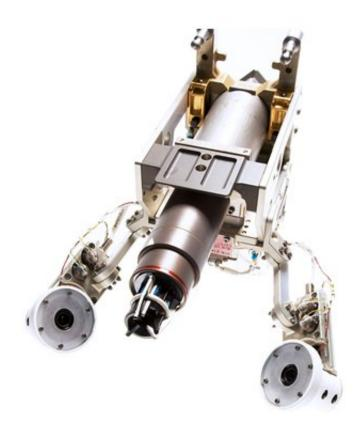
The Robotic Refueling Mission Safety Cap Tool, developed by the Satellite Servicing Capabilities Office at NASA's Goddard Space Flight Center in Greenbelt, Md. Credit: NASA
