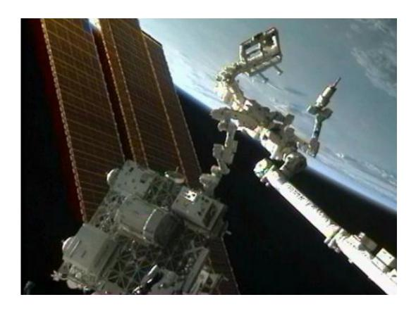
The Robotic Refueling Mission investigation (center, on platform) uses the International Space Station's Canadarm2 and the Canadian Dextre robot (right) to demonstrate satellite-servicing tasks. Credit: NASA
